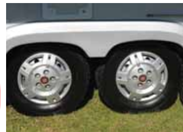
Higher load carrying capacity tandem axles
